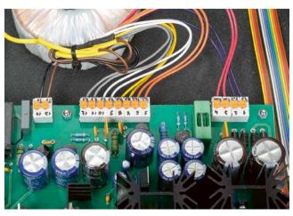
The opulent toroidal transformer is part of a sophisticated power supply system that careful tends to minimizing interference.
